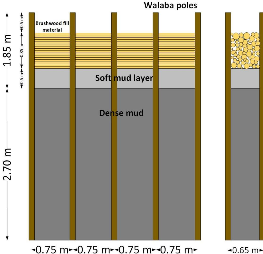
Figure 6.9 Height of poles and brushwood material and distance between the poles, front of structure and cross section respectively (Source: own illustration)
