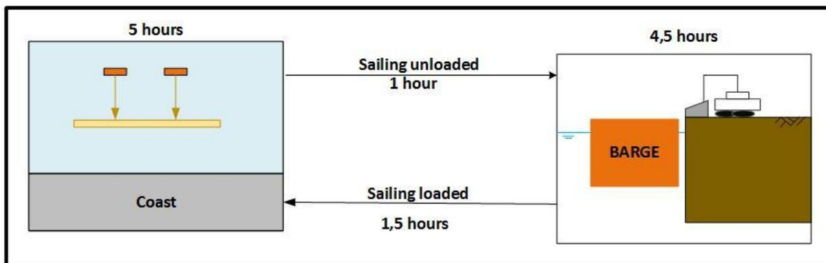
Figure 6.24 Total cycle time of the construction of the chenier (Source: own illustration)
