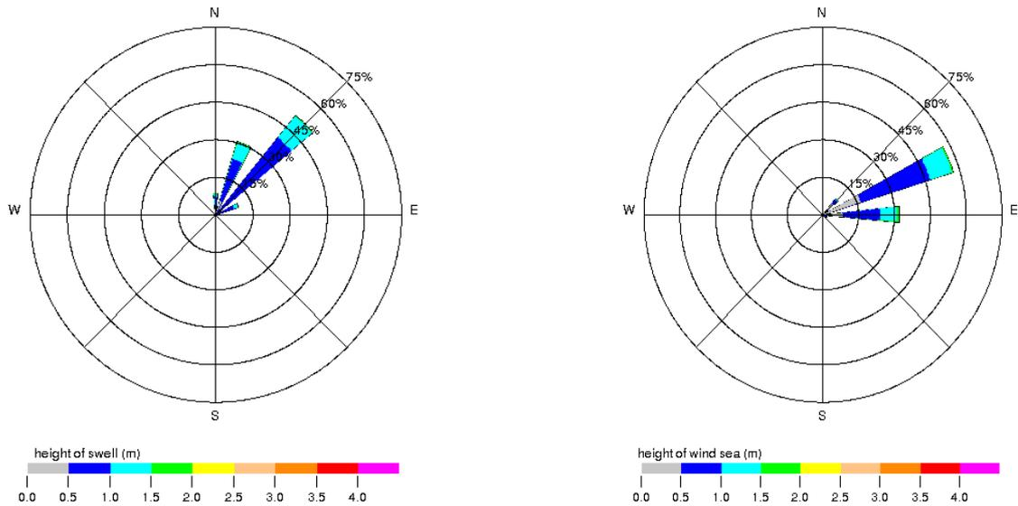
Figure B.1 Direction and height of swell and wind waves during Summer (July-September) (Source: BMT ARGOSS, 2017).
