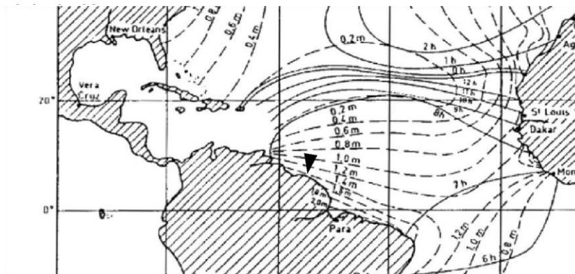
Figure 2.9 Tidal propagation in front of the coast of Paramaribo ( Bosboom et al.,2015)
