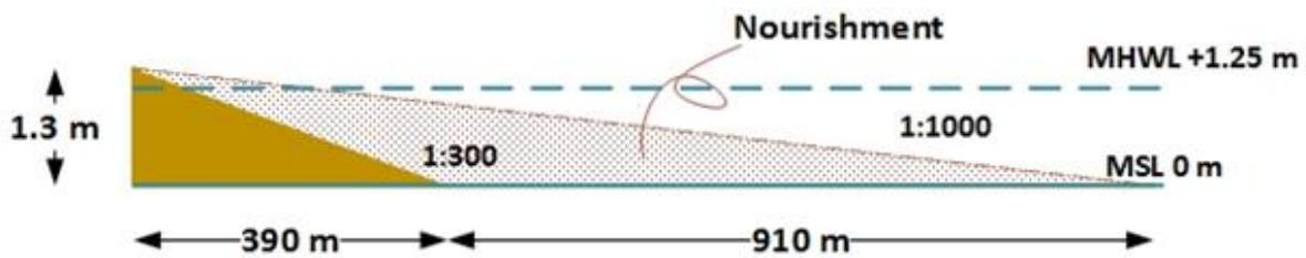
Figure 6.18 Simplified cross-sectional area of the bathymetry at WnZ and the required nourishment area (Source: own illustration)
