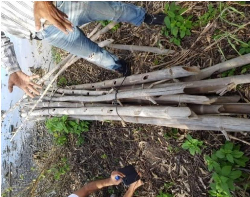
Figure 2.17 Bamboo poles with openings to prevent floating (Source: Çete, 2017)
