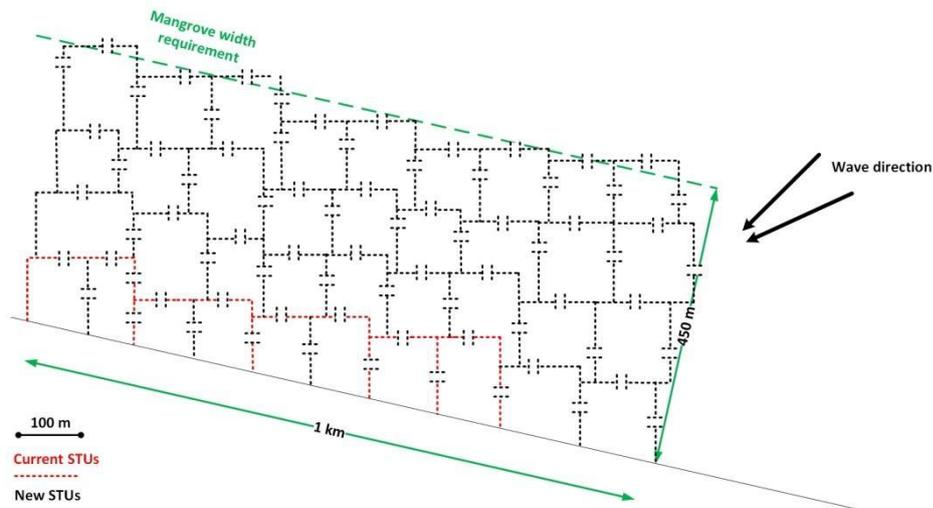
Figure 6.8 Final phase after required sedimentation in phase 2 is reached (Source: own illustration)
