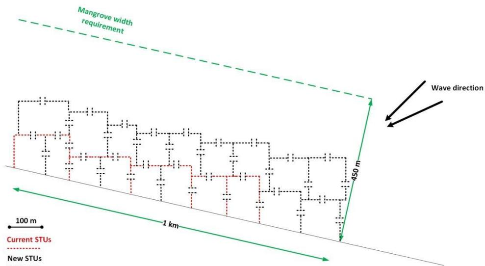
Figure 6.6 Phase 1 of construction STUs after required sedimentation in phase 0 is reached (Source: own illustration)
